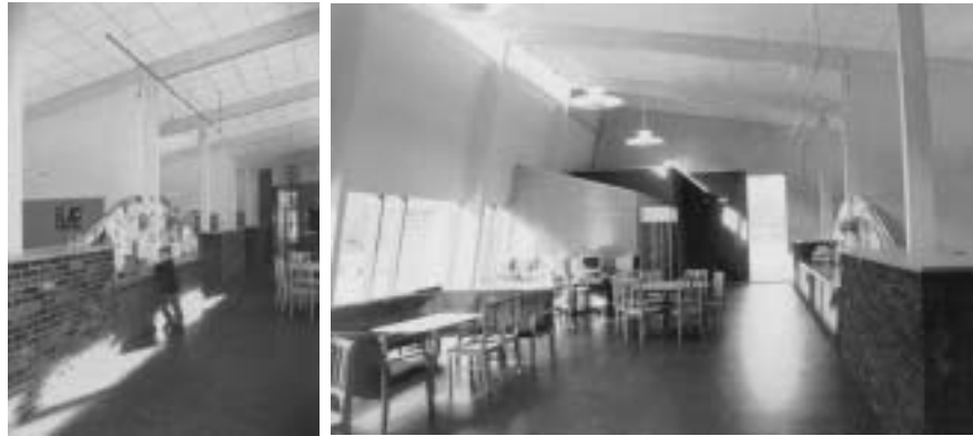
Figure 7.73 The interior of the Tredal School in Sunndalsøra, Norway is characterised by an open plan layout, a sloping roof and plenty of daylight. The ventilation inlet grills are located in the brick parapet wall separating the classrooms from the common area ( left ). The tilted roof, the window-band right under the ceiling in the west façade and the open room structure contribute in creating a strong “airy and open” spatial character ( right ).
