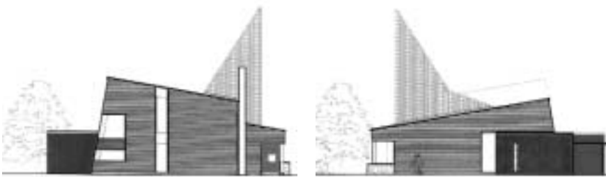
Figure 7.23 The drawings of the south façade ( left ) and the north facade ( right ) of the Tredal School illustrate that the most characteristic natural ventilation element, the extract tower, is shaped to be part of the architectural expression, and even to strengthen it. The analogy to the surrounding steep mountains is evident.
