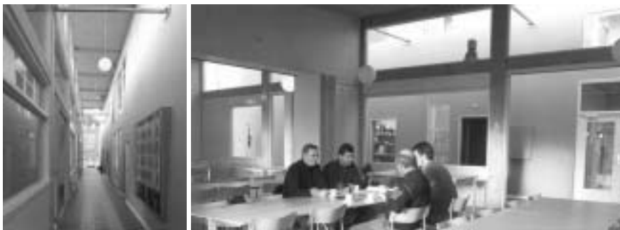
Figure 7.67 The central communication spine and exhaust stack of Kvarterhuset (community building) in Kolding, Denmark feed both the corridor ( left ) and adjacent spaces ( right ) with daylight.
