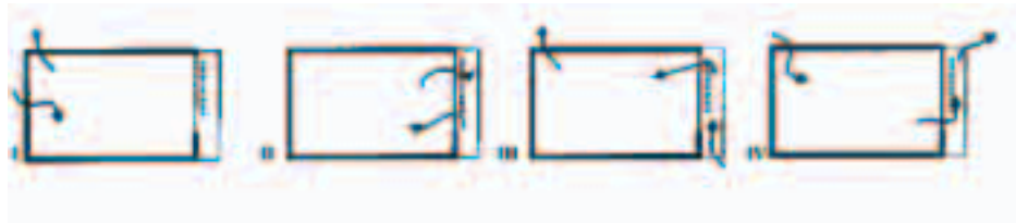
Figure 2.17 Alternative configurations for double façades 35 . I: Cavity closed. II: Cavity open. III: Cavity serving as supply path. IV: Cavity serving as extract path.
