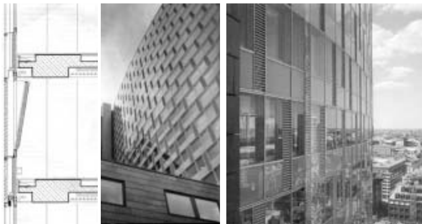
Figure 4.10 A section drawing through the east façade ( left ). The appearance of the façade viewed from street level ( middle ) and viewed from an office in the neighbouring tower ( right ).
