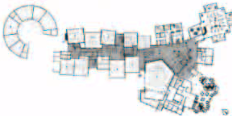
Figure 7.48 The plan of the Evangelische Gesamtschule in Gelsenkirchen, Germany is conceived as a village; the group of buildings (classrooms) are clustered around a central covered street with a public “square” at the main entrance end.
