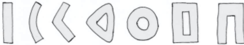
Figure 7.38 Sketches of favourable plan types for natural ventilation. Seen from left to right, the plans are simplifications of ARAG Headquarters - GSW Headquarters - Medià School, Commerzbank Headquarters - RWE Headquarters - IONICA Headquarters - and B&O Headquarters. For single-sided and cross-ventilation principles shallow plans are desired. This is most commonly achieved with a linear building form, or by wrapping the building around a closed or open courtyard.
