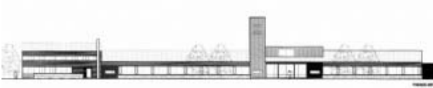
Figure 7.22 The exhaust tower of the natural ventilation concept in the Tredal School does not only affect the silhouette of the school building, but also constitutes an element of the facades. The tower accentuates the horizontality of the east façade and constitutes a focal element. The elevation of the roof to the right of the exhaust tower houses a chamber where the exhaust air is collected before it is exhausted through the tower. This chamber provides the entrance area with extra daylight through two skylight windows.
