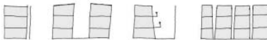
Figure 7.39 Sketch showing four typical ways of providing vertical air paths in stack ventilation: double façade/solar chimney ( far left ), atrium/central communication space ( left ), buffer zone ( right ), and chimneys/stacks that perforate a deep plan building ( far right ).
