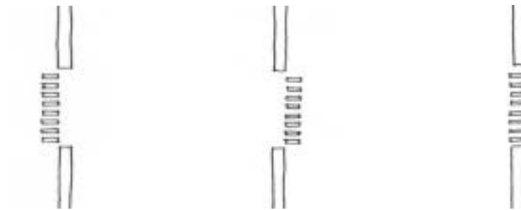
Figure 7.3 Sketches of various locations of ventilation opening components relative to the façade skin (imagine that outside is to the left). They can protrude from the façade skin ( left ), be set back into the façade skin ( middle ), or be aligned with the facade skin ( right ). Key words include relief, depth, light, and shadow.
