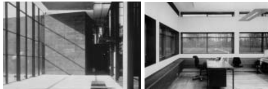
Figure 7.70 Daylight is introduced in various ways and amounts in the Pihl & Søn's Headquarters, and the floor-to-ceiling height of the interior spaces varies from one to three stories ( left ). Skylight windows provide the offices with fresh air and daylight deep into the spaces ( right ). Simplicity in the choice of materials and high quality finishing is conspicuous in the expression of the building, both in the exterior and in the interior. The materials chosen; natural stone, brick, solid wood and steel need little maintenance and have a long lifespan. These materials are also associated with low emission, and stone and brick have high thermal mass. The natural colours of the materials -black, white and grey-are neutral and "classical colours". The architects wanted the building to form a neutral background for the occupant's personal character through e.g. pictures and objects.
