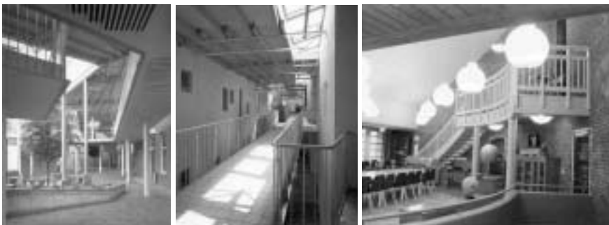
Figure 7.76 The unheated indoor street space in the Eveangelische Gesamtschule in Gelsenkirchen, Germany is used as a climatic buffer with cold air arriving through embedded ducts at the bottom and warm air escaping at the top ( left and middle ). The interiors of the Jaer School in Nesodden, Norway is characterised by the extensive use of brick (thermal mass) and a varying floor-to-ceiling height in some of the spaces. The outlet into the extract chimney can be seen high up on the wall in the media hall ( right ).
