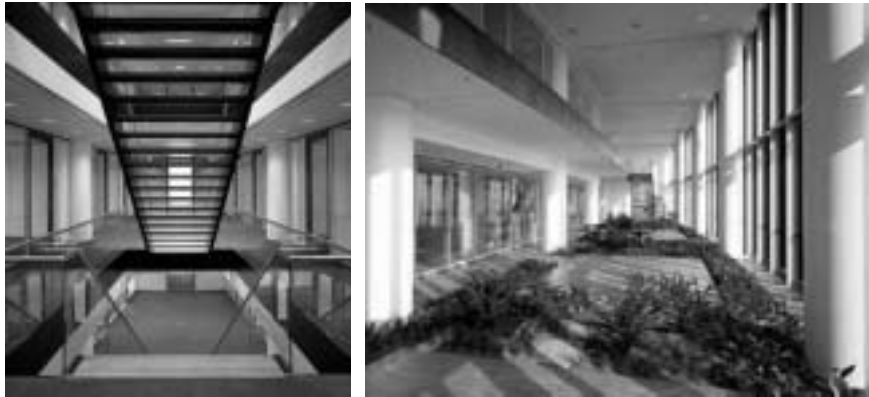
Figure 7.71 The office floors of the ARAG Headquarters in Düsseldorf, Germany are simple and open in feel, and the shallow plan is provided with daylight from two sides ( left ). Cellular offices and meeting rooms ring the perimeter while group-meeting spaces occupy the centre of the lens-shaped plan. The narrow shape of the plan makes utilisation of daylight possible also in the core of the building, and a view to the exterior is provided from all working desks. The double-height “sky-gardens” provide lungs of air and light on every eighth floor ( right ). Planted with “meadows” of tall grass and wild flowers, the gardens provide informal meeting areas and relaxation spaces.
