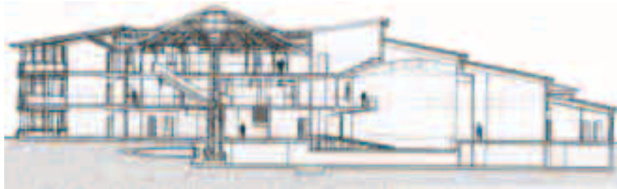
Figure 7.44 The section drawing of the Waldorf School in Cologne, Germany shows the build-up of volumes in height towards the central outlet located in the roof of the luminous volume of the central hall at the heart of the school.
