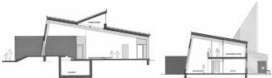
Figure 7.55 Cross section through the entrance area of Tredal School showing the embedded supply duct and the extract chamber with integrated skylights( left ). Cross-section through the two-storied administration block in the southern end of the linear building volume ( right ).
