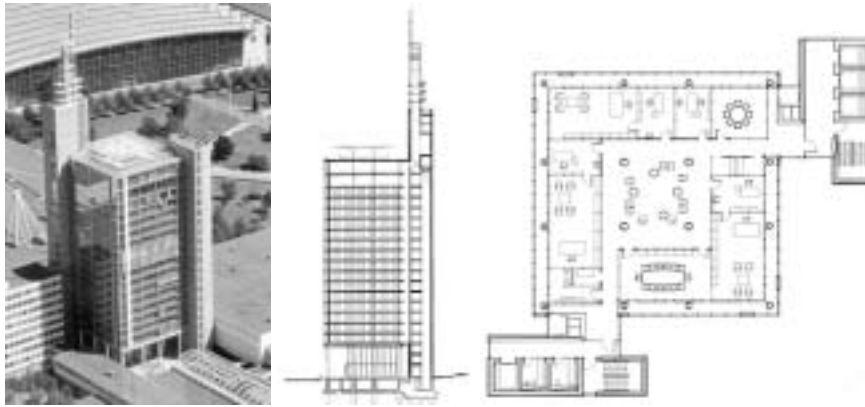
Figure 3 The administration building of Deutsche Messe AG is widely visible on the exhibition area in Hanover, both because of its height compared to the neighbouring exhibition halls and because of the ventilation chimney stretching up towards the sky ( left ). Drawing of the section ( middle ) and drawing of the plan with offices located along the facades and meeting/group rooms in the core ( right ).
