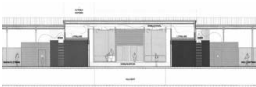
Figure 7.56 Lengthwise section through the entrance area in the Tredal School showing the extract chamber that extends over the central part of the building and its main entrance only. This is different from the Mediå School in Grong, Norway where the extract chamber runs the whole length of the plan. The section drawing above also shows the generously sized supply duct embedded under the building.
