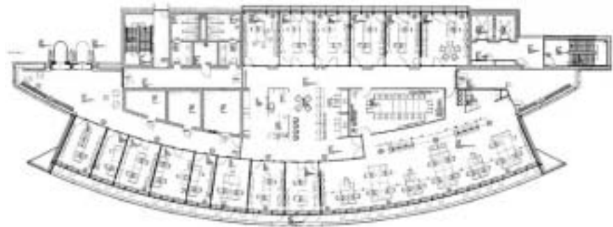
Figure 7.46 The plan of the MDR-Zentrale in Leipzig, Germany is double banked with the offices along the facades and meeting rooms and service functions in the core. The curvilinear double south façade is one of the most characteristic features of the building.
