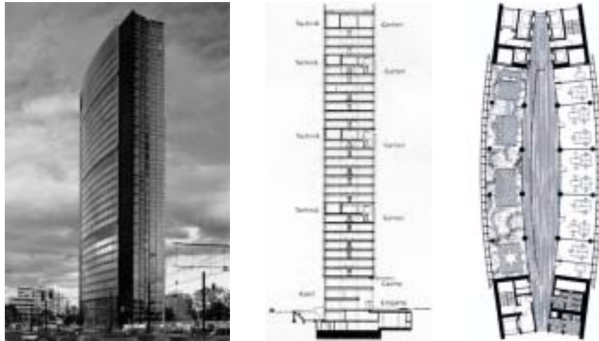
Figure 20 The slender proportion of the high-rise building of the ARAG Headquarters is not unlike that of the GSW high-rise in Berlin ( left ). Drawing of the section ( middle ) and drawing of the plan ( right ).
